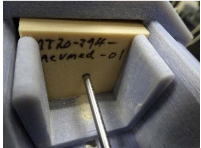
Figure 4 Post-test Acumed Acutrak 2 specimen fully inserted, the proximal end flush with the foam surface.
