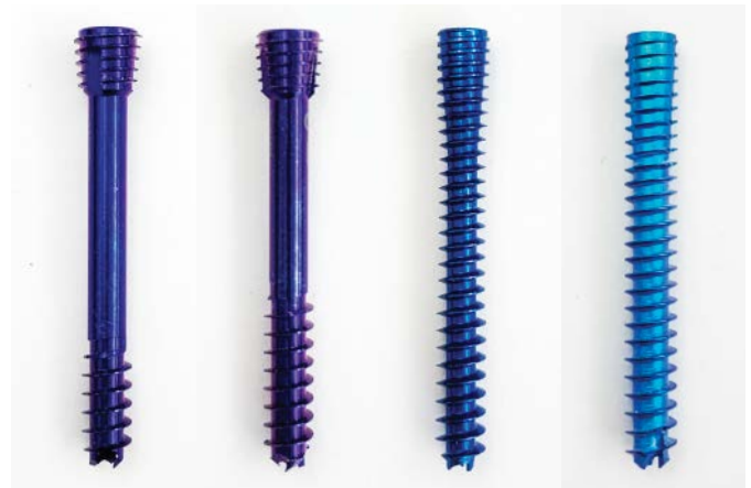
Figure 1 Representative screws tested (left to right): DePuy Synthes CCHS Short Thread, DePuy Synthes CCHS Long Thread, Acumed Acutrak 2, Arthrex Compression FT.
