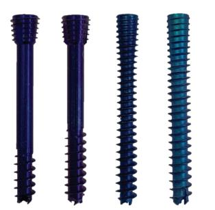
Figure 1 Representative Screws Tested (left to right): DePuy Synthes CCHS Short Thread, DePuy Synthes CCHS Long Thread, Acumed Acutrak 2, Arthrex Compression FT
