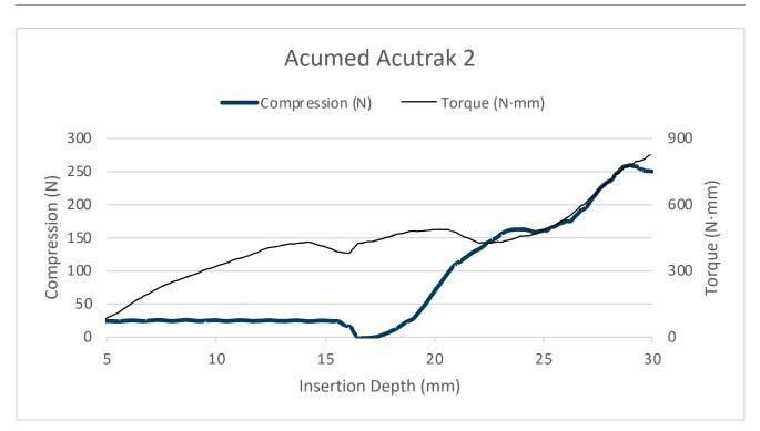
Figure 7 Representative Acutrak 2 Compression and Torque Performance
