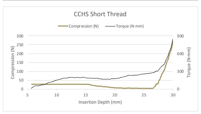
Figure 5 Representative CCHS ST Compression and Torque Performance
