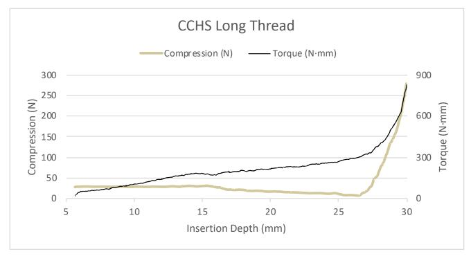
Figure 6 Representative CCHS LT Compression and Torque Performance
