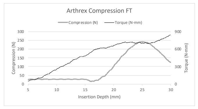
Figure 8 Representative Arthrex Compression FT Compression and Torque Performance
