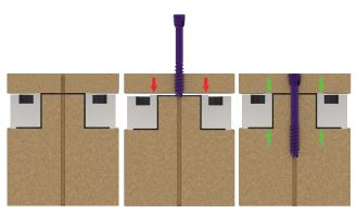
**Figure 2** Midline fracture setup with no initial fracture gap (left), screw cutting into distal block (middle), and fully inserted screw (right). Load cell shown in silver.
