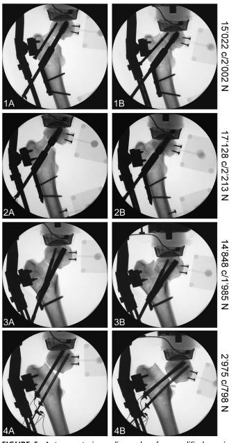
**FIGURE 5.** Anteroposterior radiographs of exemplified specimens in the 4 groups (1: DHS-screw; 2: DHS-blade; 3: FNS; 4: 3CS) before testing (1A, 2A, 3A, 4A) and after failure onset (1B, 2B, 3B, 4B). The number of cycles to failure onset and the respective load at failure are shown on the right hand side. Shortening of the femoral neck/leg and varus tilting are visible looking at each specimen's head marker sets.
