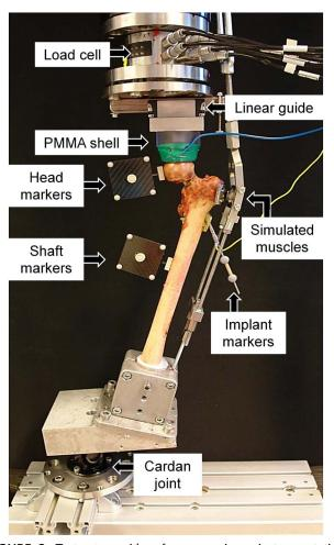
**FIGURE 2.** Test setup with a femur specimen instrumentation with FNS, equipped with retro-reflective markers for optical motion tracking and mounted for biomechanical testing. **Editor's Note:** A color image accompanies the online version of this article.
