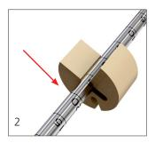
Insert the appropriate length variable angle locking screw.
